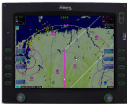
Figure 1 – Avidyne FlightMax EX-Series 700-00004-XXX-()
